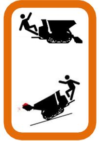
**Caution:** Ensure that the shovel, if equipped, is in its full up position before dumping. If the shovel is down while dumping the shovel will contact the ground making the machine unstable and unable to dump. Never dump the machine on a declining slope. Look for barriers when dumping and never run the machine too quickly when moving or turning.
