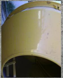
10) TK poly drum mixers are made of durable 1/2" polyethylene, making the clean-up effort much easier and less time-consuming. These same mixers come with 6 easy to replace mixing blades bolted onto the drum.
