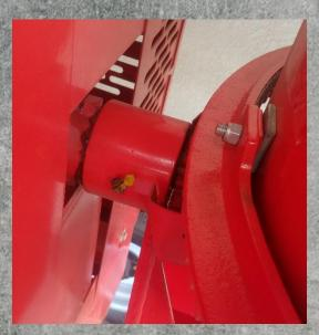
5) TK's one-piece cast-iron ring gear is securely bolted to the drum compared to ring gears that are gapped away from the drum or are made of multiple pieces. This design allows for smoother drum rotation, reduces noise and lessens the chance of the gear ring coming loose during operation.
