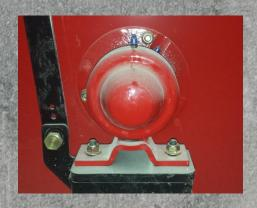
2) Unlike other mixers, the engagement handle on TK mortar mixers are routed through the frame tube to protect it from dust, mortar, weather related issues, and forklift damage and it is located on the front leg for easier operation when dumping the mix.
