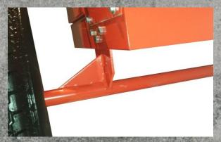
6) We use a welded grid in our mixer compared with electric heat welding grids which typically do not last as long.
