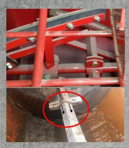
8) We use spring loaded steel latches for longer life vs. rubber hood latches that become brittle due to exposure to weather.
