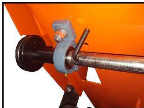
Hinged guard with easy lock for arbor replacemnet
